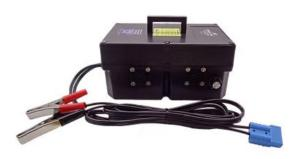
Constant voltage regulation. Allows the regulation of the flow rate of the 12 Volt pumps. Includes anti-polarity change protection and thermal protection. Pump stop system. It can be regulated under flow rate up to 40 ml/min.For MEGA-MONSOON pump.
