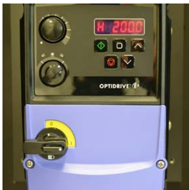
Fig. 8d Switch 3 set to 200 Hz
