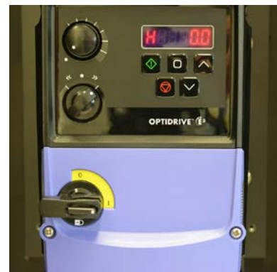
Fig. 8c Switch 2 set to >> forward
