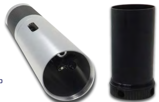
Measurement chamber removed from probe sleeve
