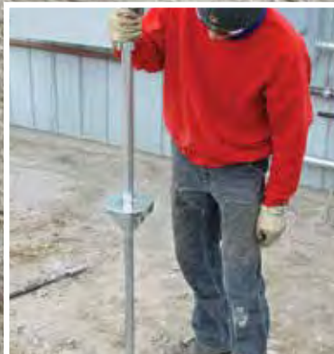
Dynamic cone penetrometer (part# 59000) can evaluate strength and density of soil, in situ.
