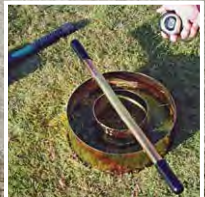
Infiltration rings (part# 400.97) can monitor infiltration rates, and study liquid waste disposal, leaching, and drainage efficiencies.
